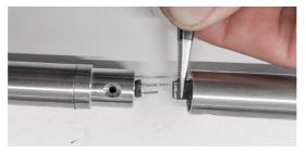
Now insert the connector of the extension into the socket of the basic unit. (The socket can be held with tweezers, for example.) Make sure that the connector is pushed all the way into the socket.
